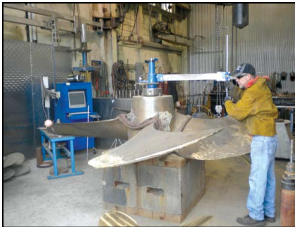
Inside the Shop: Todd Simpson uses the Pitchometer for measuring the geometry of propellers.
