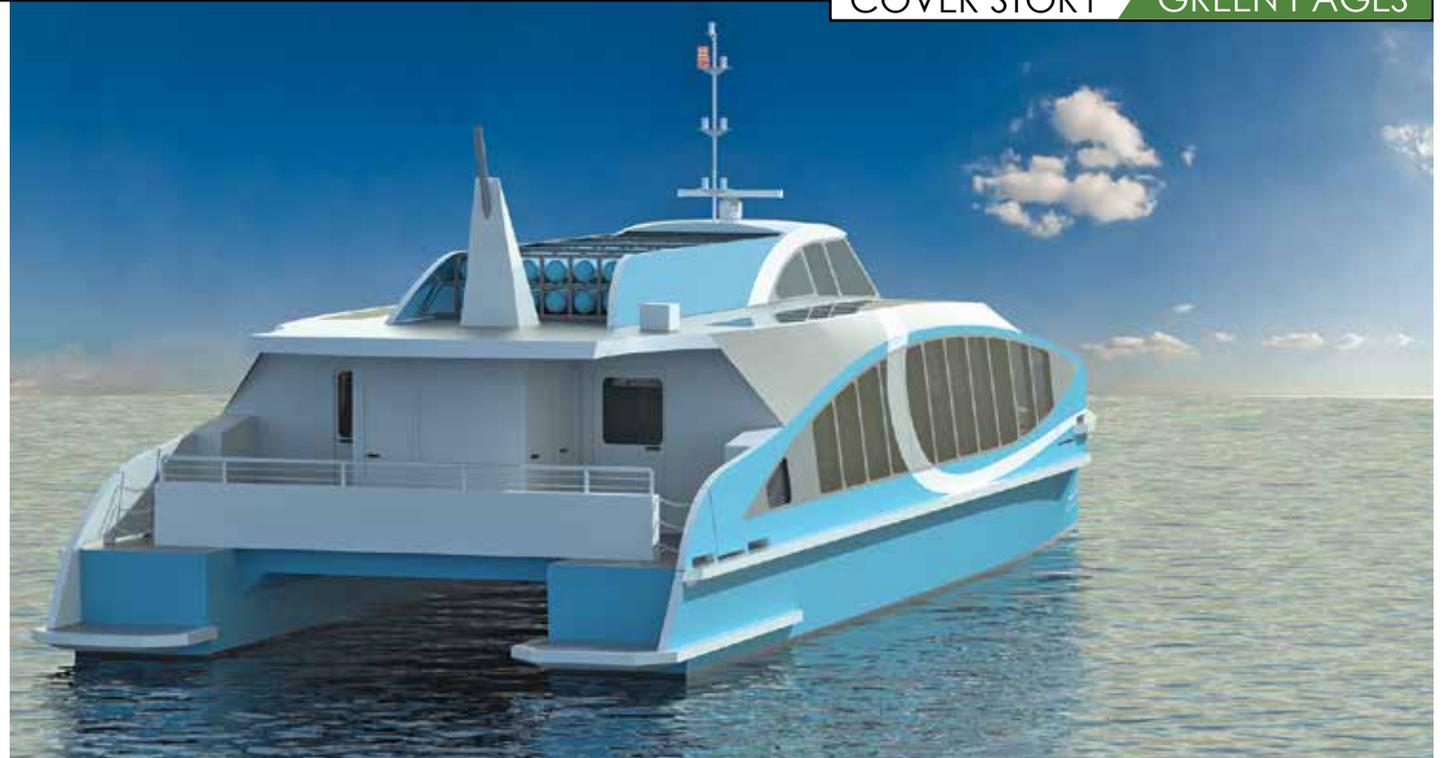
The 70-foot-long, all-aluminum Water-Go-Round will carry up to 84 passengers at a top speed of 22 knots.
