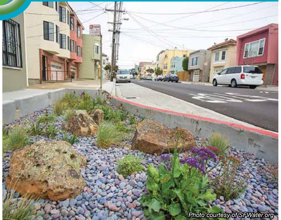
*Planted bulb-outs and rain gardens constructed on a nine-block stretch of San Francisco's Holloway Street now provide a way of keeping stormwater out of the sewer system by capturing it upstream.*
