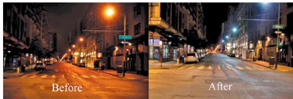
Once the 14-month-long, $16 million LED streetlight conversion project is completed, San Franciscans will notice dramatically improved nighttime lighting. LED output has been compared to the natural light of the moon.
