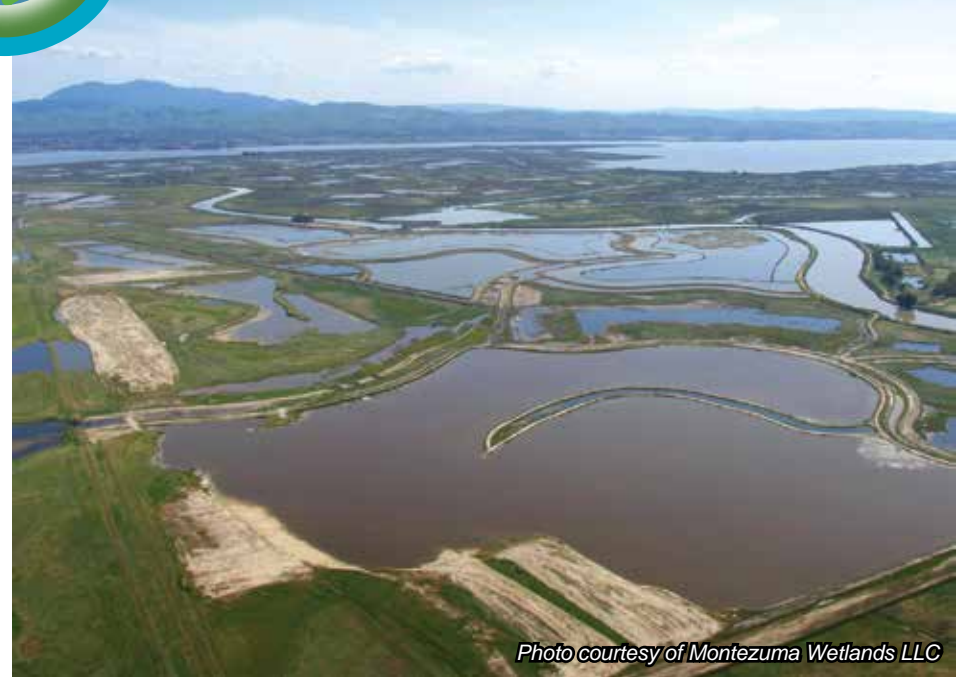
Recently, 400,000 cubic yards of sediment were deposited at the Montezuma wetlands near Suisun Bay to help restore the threatened native habitat of endangered fish and wildlife.
