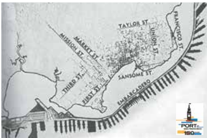
The Great Seawall was constructed 1878 - 1915. More than three miles long, it created over 700 acres of new land that was previously under water.
