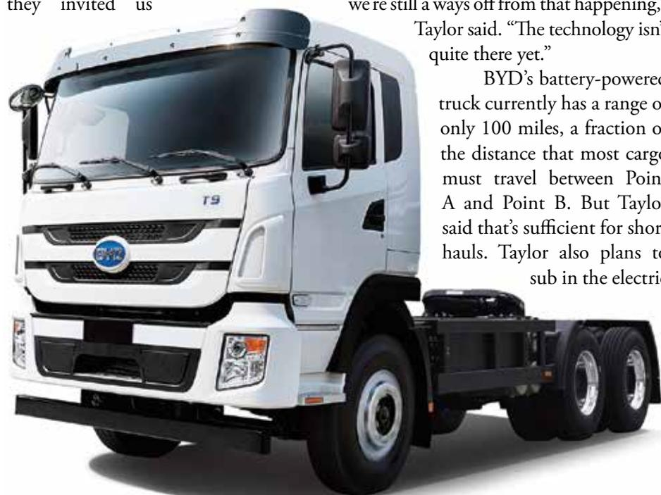
Manufacturer BYD wants to prove that zero-emission, battery-powered trucks can be used in heavy-duty applications. The current range of their battery-powered truck is 100 miles.
